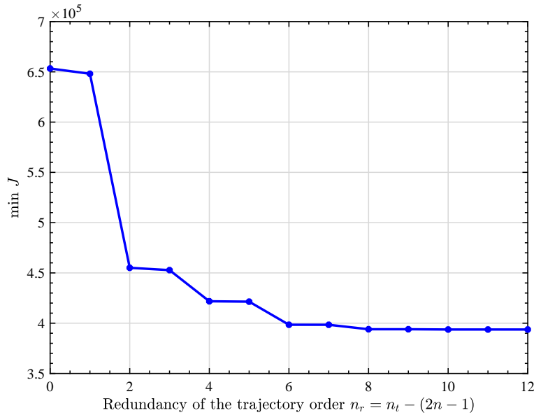
Figure 3.13 Relationship between the minimum value of J and the redundancy of the trajectory order n_r in (3.7) ( t_{pa} = -2.4\tau ).
